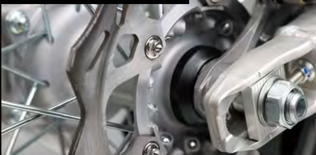
Rear DISC BOLT ( KX450F ) Thin Head 10 mm - M8 x 14.5 ZT31-3724
