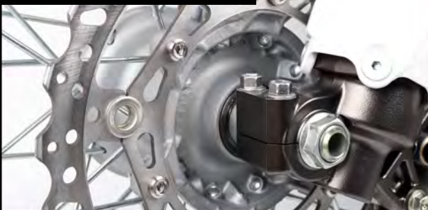
Rear DISC BOLT ( KX450F ) Thin Head 10 mm - M8 x 14.5 ZT31-3724
