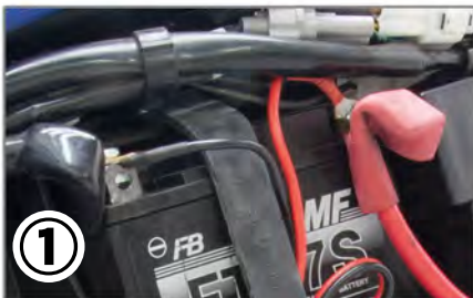
① Install the battery charging harness to your bike.
